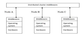
Fig. 6 Cluster Based Software Architecture
