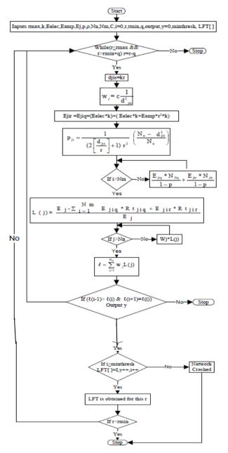
Fig. 8 Proposed Placement Algorithm
